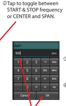
③ Enter desired frequency on keypad, select units (MHz, GHz, etc.).
