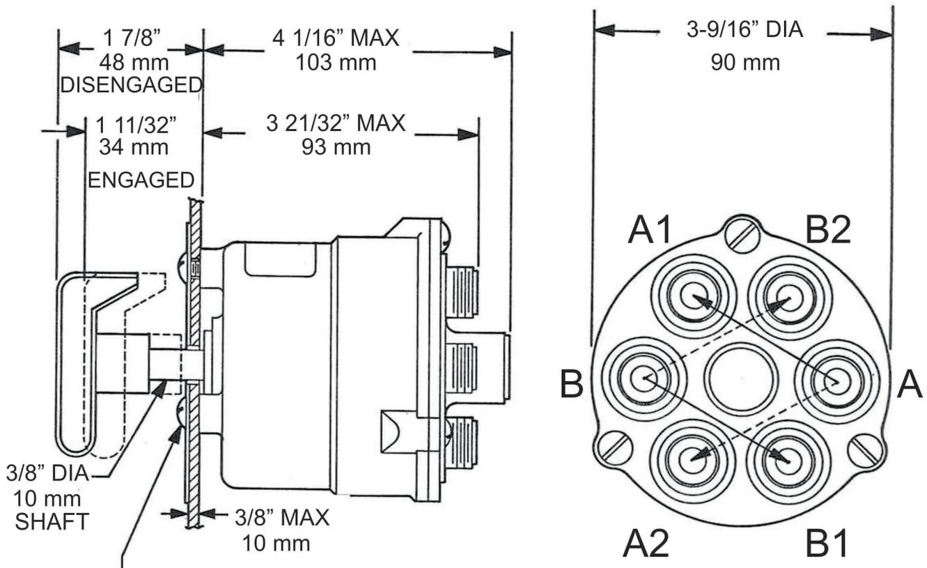
MOUNTING DIMENSIONS  $\frac{7}{32}$ " (6 mm) MTG HOLES FOR THREE 10-32 SCREWS SPACED AT  $120^\circ$  ON  $1 \frac{1}{4}$ " (32 mm) RADIUS
