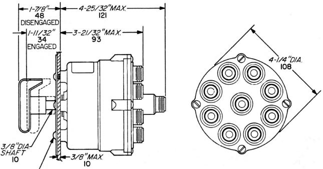
MOUNTING DIMENSIONS: 7/32"(6mm) MTG. HOLES FOR FOUR 10-32 SCREWS SPACED AT 90° ON 1-5/16"(33mm) RADIUS
