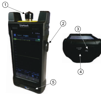
Figure 1 SK-9000 Controls, Indicators, Connectors and Ports
