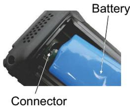
3. Connect new battery cable to connector in the battery compartment.
