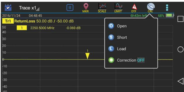
Match measurement verifies and monitors the match conditions in the antenna system at various frequencies. The results are shown on an x-y graph. Frequency is shown on the x-axis and Return Loss or SWR is shown on the y-axis.
