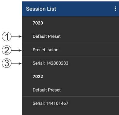
When a power sensor is connected to the Bird RF Meter the first time the Generic Session File (Default Preset if created) is used to initialize the App then a Serial Number Specific Session File is automatically created.
