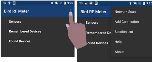
**Network Scan** — This menu option scans the WiFi network the android device is connected to for any Bird devices connected to the same network.
