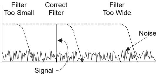
Except for average power and VSWR measurements, all WPS measurements rely on a variable video filter to improve accuracy. This filter can be set to either 4.5 kHz, 400 kHz, or full bandwidth (10000kHz). It should be as narrow as possible while still being larger than the demodulated signal bandwidth (video bandwidth). Narrowing the filter limits the noise contribution caused by interfering signals. Listed below are some common modulation schemes and the appropriate video filter.
