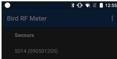
7. Tap the Power Sensor model number to connect to the Power Sensor.
