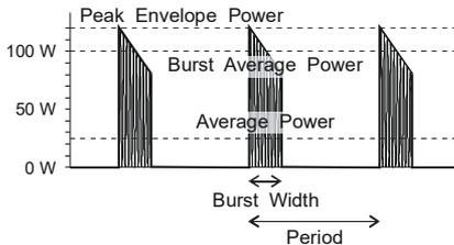
Burst width (BW) is the duration of a pulse. Period (P) is the time from the start of one pulse to the start of the next pulse. Duty cycle (D) is the percentage of time that the transmitter is on. To calculate the duty cycle simply divide the burst width by the period ( $D = BW / P$ ). Low duty cycles mean that the burst width is much less than the period; a large amount of dead time surrounds each burst. For low duty cycles, the burst average power will be much larger than the average power.
