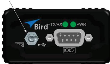
2. Connect a USB cable between the 4421B540-2 and the computer.
