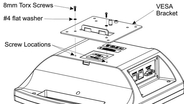
3. Insert the screws into the washers, then drive screws into the indented holes on the rear of the 4421A. The screw will break through a thin plastic barrier.
