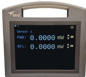
**One Sensor Operation** — The 4421A RF Power Meter will display the RF power measurements of one RF Power Sensor. The sensor may be connected to either of the Sensor connectors, see ["4421A Controls and Indicators" on page 6](#).
