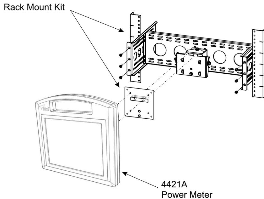
After the Rack Mounting kit is installed in a rack, the 4421A can be removed and reinstalled without the use of any tools.
