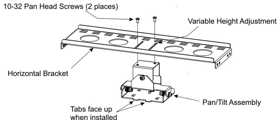
2. Position the Horizontal Bracket over the Pan/Tilt Assembly.
