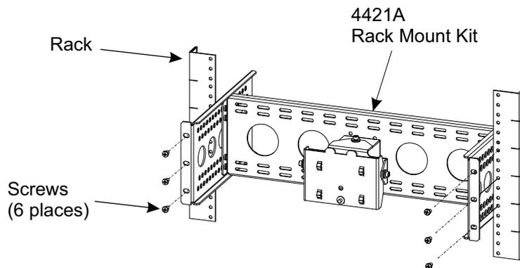
The Rack Hardware Kit provides various screws and nuts for the four most common types of racks.
