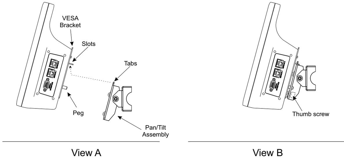
2. Insert the peg on the VESA Mount into the hole on the Pan/Tilt Assembly.
