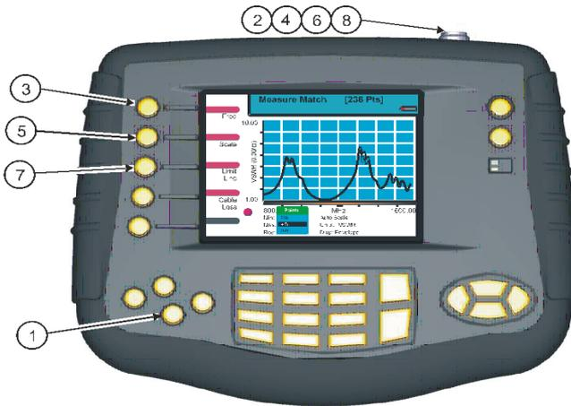
Match measurement verifies and monitors the match conditions in the antenna system at various frequencies. The results are shown on an x-y graph. Frequency is shown on the x-axis and return loss, cable loss, or VSWR is shown on the y-axis.
