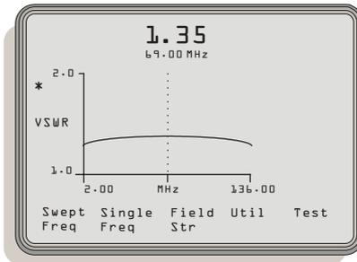
In the single frequency mode Auto Scaling sets the measurement unit scale so the pointer is mid range of the previous reading. The maximum and minimum scale values are approximately 10% higher or lower than the measured value.
