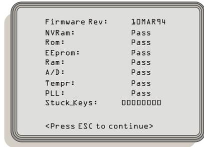
Firmware Rev—Revision date for the firmware installed.
