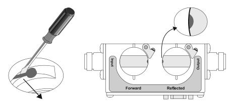
3. If the contact is accidently moved too far, the element will not slide into the socket. Move the contact back into the recessed area and repeat the process.
