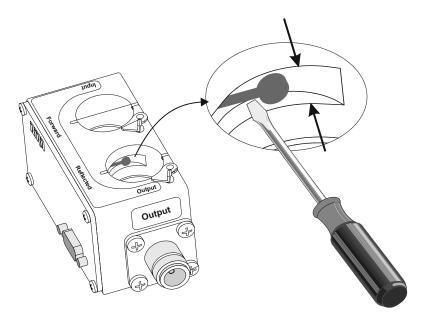
2. After centering the contact, bend the contact bar slightly toward the center of the element socket bore, so that the profile of the element contact is visible when viewing the element socket from the top of the socket bore.
