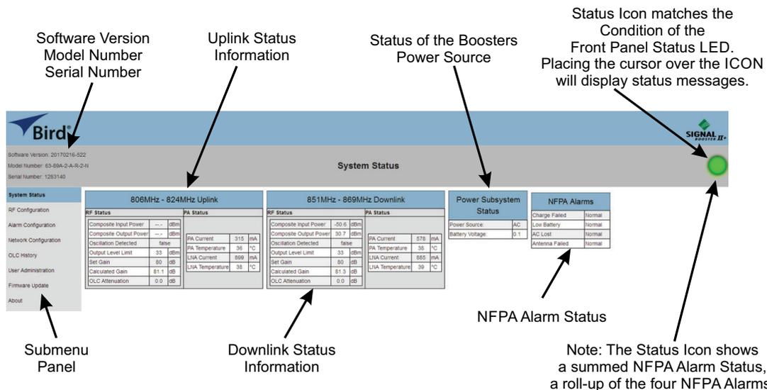
On the left-hand side of the page is a panel containing the major submenus available to the user including System Status, RF Configuration, Alarm Configuration, Network Configuration, OLC History, User Administration, and Firmware Update. Place your cursor over a particular submenu heading and left click to make a selection. Each major submenu page contains a group of related functions and each is discussed in detail in later sections of this manual.
