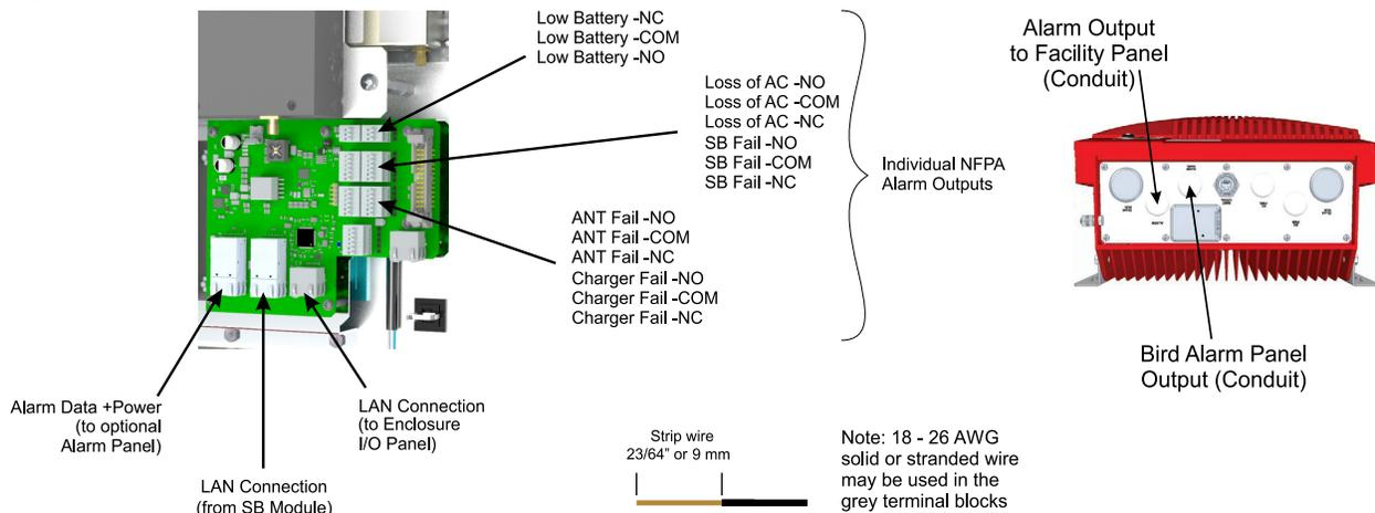
Figure 46 Battery Backup and Facility Fire Panel Integration
