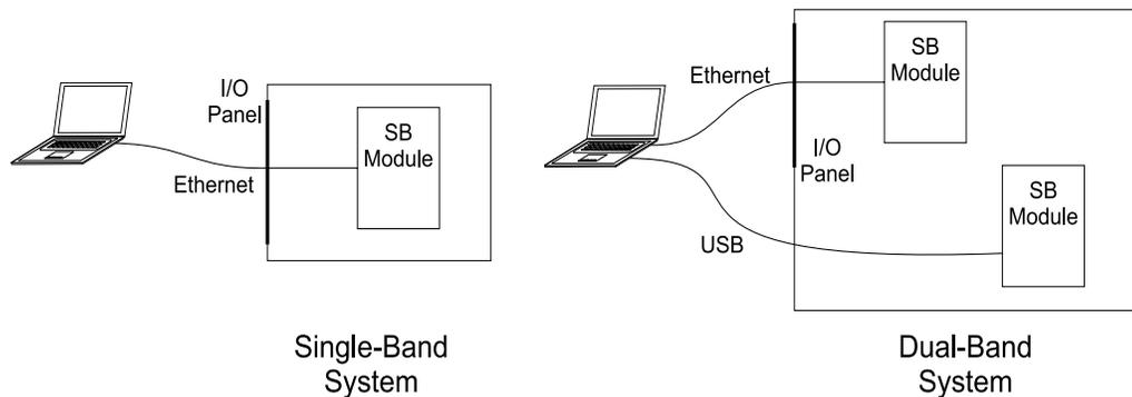
The advantage of the Ethernet connection is the chassis need not be opened to accomplish a firmware update. On dual-band systems the chassis must be opened to access the USB port on the second SB Module.
