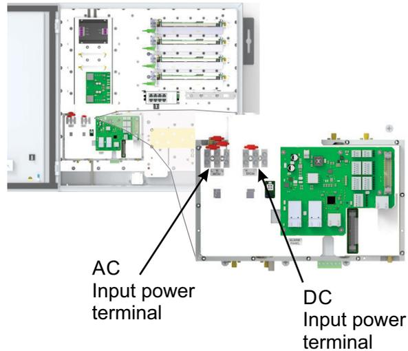
All Fiber-DAS Remote units have the AC and DC input terminals located on the left end of a panel in the bottom portion of the enclosure, see [Figure 38](#).
