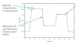
State average measurements allow you to capture the stable region of up to 4 states within multilevel pulses
