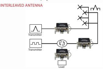
HD Radio and an analog signal can use interleaved antennas for separate but simultaneous transmission. High isolation reduces the mutual coupling however, analog power coupled to the digital transmitter must be considered when specifying the BPME. With 20 dB of dynamic range, the BPME is ready to handle this type of installation.
